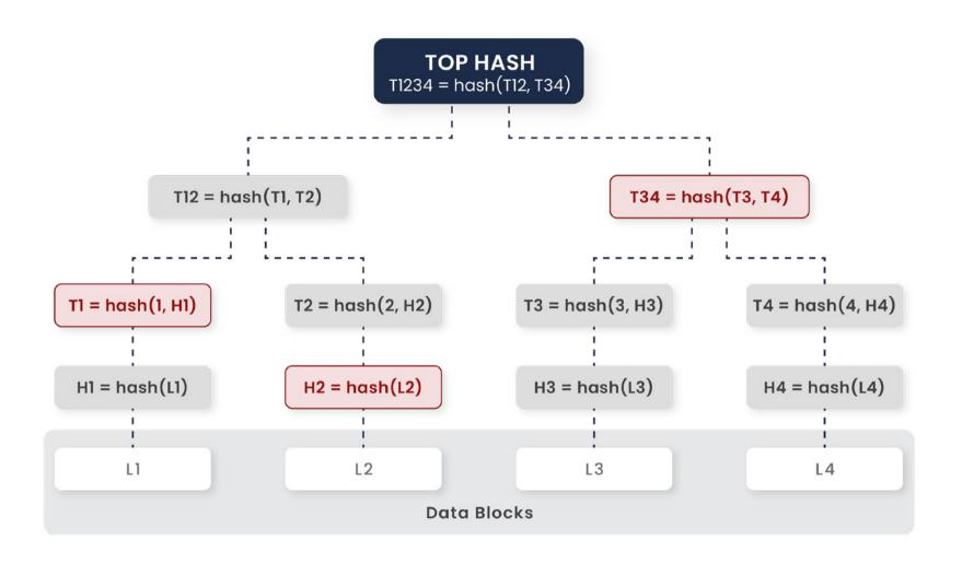
In AIOZ CDN, a complete merkle root tree of a video segment which is being stored in Worker Nodes could be constructed from different hashes, with one hash per level being sufficient (Figure). From this tree, HUB Node will get the final TOP HASH of which size is log2(X) (X is the number of nodes in the tree).
