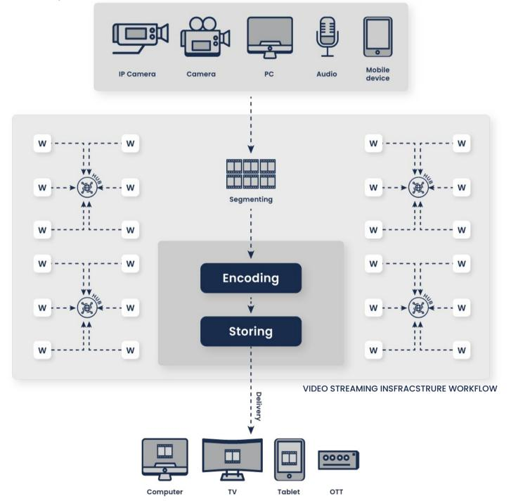
Figure. Overall workflow of AIOZ CDN
