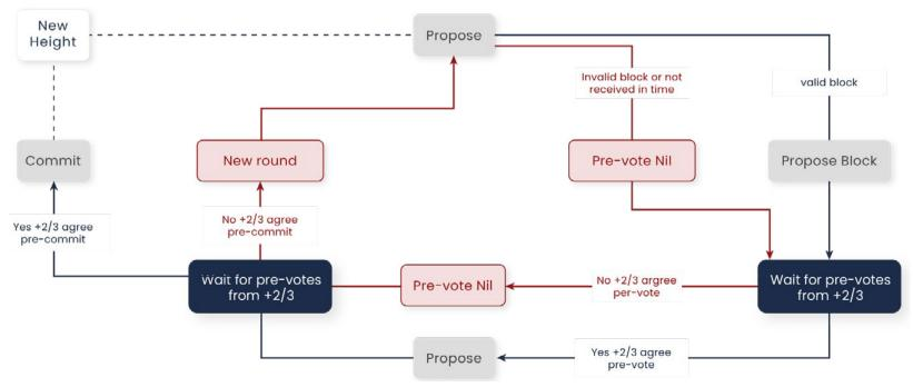
The block proposing process is summarized in Figure : Validators take turns proposing blocks for the transaction and voting on the proposed blocks. The blocks are submitted to the chain with each block on the chain at each height. However, the block may also fail to submit. In this case, the protocol will select the next certifier to propose a new block at the same height and start voting again.
