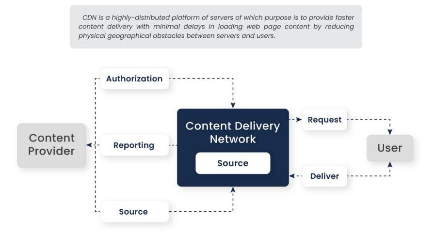
Figure. Model of a typical CDN
