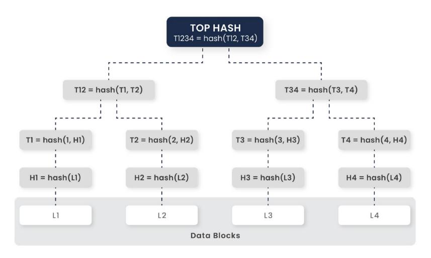
The illustration for a typical Merkle root in AIOZ CDN is shown in Figure. Instead of only 4 blocks shown in Figure, in reality, a video segment contains n blocks, which n is computed so that the size of each block ranges from 32 to 64 bits. Via gradual pairing, we will finally achieve a TOP HASH, which is unique for one video segment. In other words, either any changes in any blocks or any block disorders of a video segment will lead to a totally different TOP HASH.
